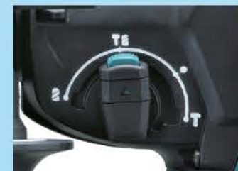
3 mode operation Rotation + Hammering / Hammering only / Rotation only
