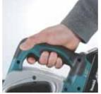
**Rubberized soft grip** Handle is widely covered with elastomer for more comfort. control and less fatigue.
