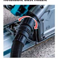
Added two leaf springs enable to twist and lock the nozzle with a click in order to reduce unexpected rotation.
