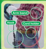
Protection of extension cord from breakage
