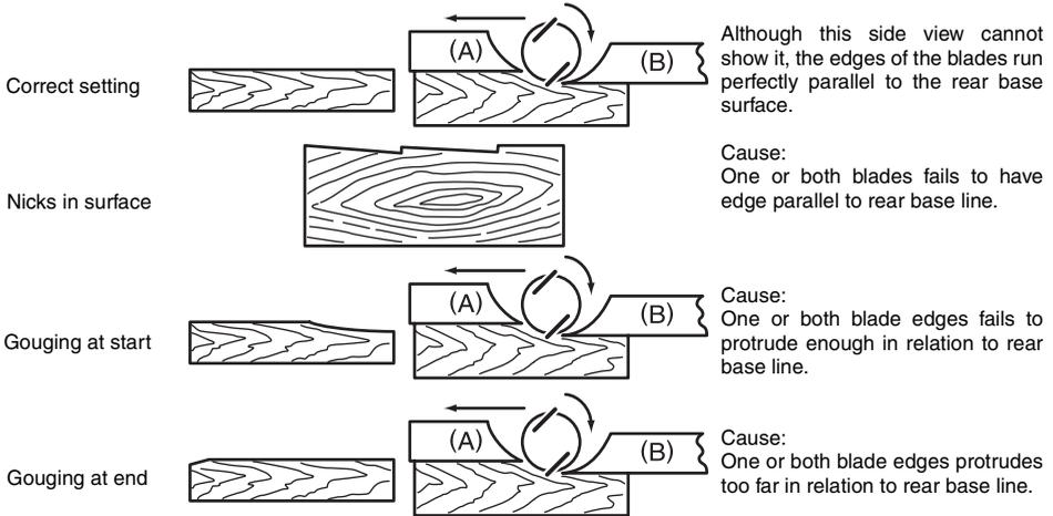
**Adjusting the depth of cut (Fig. 6)**
