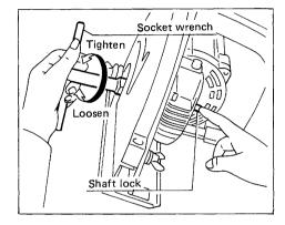
To install the wheel, follow the removal procedure in reverse.
