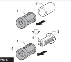
1. Prefilter 2. Tubular sponge filter 3. Mesh pipe 4. Guide stoppers 5. Guide hole
