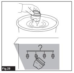
NOTE: Avoid fastening the attachment end (rubber sealing ring) of high performance filter when hanging it up for drying.
