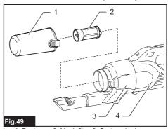
1. Dust case 2. Mesh filter 3. Cyclone body
