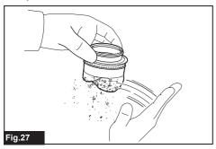
Wash the high performance filter in soapy water when it is clogged with dust and dirt. Dry it out thoroughly in the shade before use.
