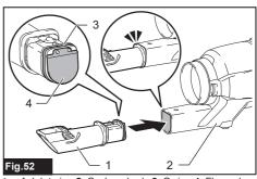
▶ 1. Inlet pipe 2. Cyclone body 3. O-ring 4. Flap valve
