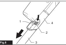
1. Release button 2. Arm of release button 3. Attachment with lock function 4. Suction inlet
