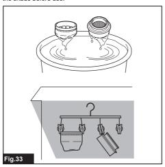
**NOTE:** Avoid fastening the attachment end (rubber sealing ring) of HEPA filter when hanging it up for drying.
