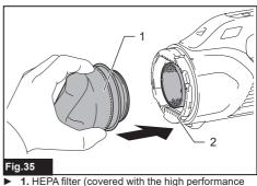
1. HEPA filter (covered with the high performance prefilter)
