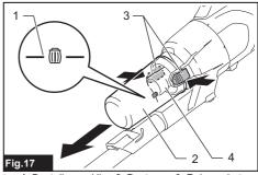
1. Dust disposal line 2. Dust case 3. Release buttons 4. Mesh filter
