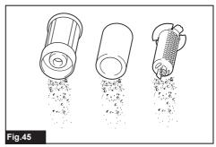
5. Wash the filters and mesh pipe in soapy water when they are clogged with dust and dirt. Dry them out thoroughly in the shade before use.
