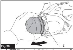
1. HEPA filter (covered with high performance prefilter) 2. Cleaner body
