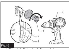
▶ 1. Side grip 2. Protrusion 3. Groove 4. Arm
