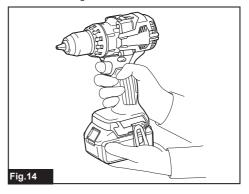
**NOTICE:** Do not cover vents, or it may cause overheating and damage to the tool.
