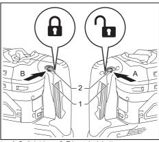
▶ 1. Switch trigger 2. Trigger-lock button
