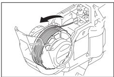
**8.** Release the lock lever. The release lever returns, and the wire is held by the left and right gears.
