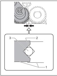
1. Gear 2. Path of the wire 3. Wire
