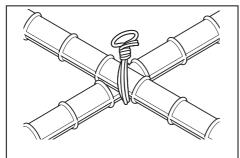
If tying strength is insufficient, change the tying orientation and perform tying twice so that tying strength increases.
