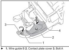
1. Wire guide B 2. Contact plate cover 3. Bolt A
