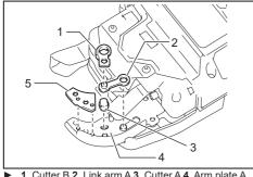
1. Cutter B 2. Link arm A 3. Cutter A 4. Arm plate A
