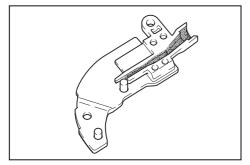
**5.** Remove cutter A, cutter B, top plate, and link arm A from arm plate A. Then, clean them.
