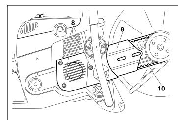
Unscrew the screws  $({\bf 8})$  and remove the crankcase housing cover  $({\bf 9}).$
