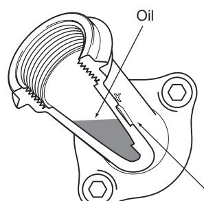
The oil is visible from here, so the MAX and MIN marks can be used to check the quantity of oil.
