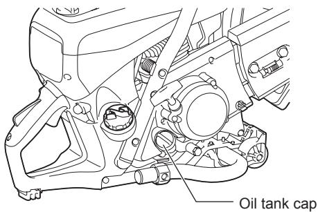
(1) Place engine on the level and remove oil cap.
