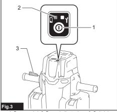
▶ 1. Power switch 2. Power indicator lamp 3. Switch lever
