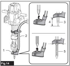
1. Dust cover 2. Hose 3. Bit with collar 4. 30 mm -100 mm 5. Bit without collar
