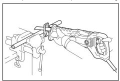
**NOTICE:** Do not cut the workpiece with the shoe away from the workpiece or without the shoe. Doing so increases the reaction force which may break the recipro saw blade.
