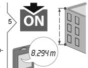
The result is shown in the main line and the measured distance above.
