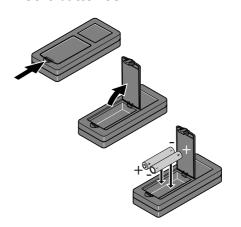
To ensure a reliable use, do not use zinc-carbon batteries.
