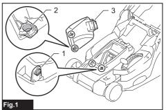
Protrusion 2. Hole 3. Battery cover
