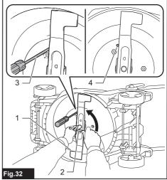
▶ 1. Mower blade 2. Wrench 3. Screwdriver 4. Hole
