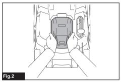
**3.** Make sure that the battery cover is attached securely, and the battery cover is locked securely with the locking lever.
