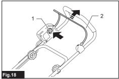
3. Release the switch lever to stop the motor.
