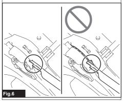
2. Align the hole in the upper handle with the hole in the lower handle, then insert the bolt from outside, and then tighten the thumb nut from inside. Perform the same procedure on the other side.
