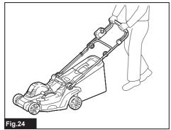
NOTE: When cutting long lawn or dense lawn, if the unevenness in the length of lawn or poor finish is found after mowing, or decrease of the motor speed is found during mowing, decrease the mowing speed lower than recommended in this manual, or raise the mowing height. The center lines of the front wheels are guidelines to mowing width. Using the center lines as guidelines, mow in strips. Overlap by one half to one third the previous strip to mow the lawn evenly.
