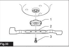
1. Blade support 2. Mower blade 3. Bolt
