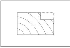
To make a stepped cut as shown in the figure, use the edge fence (guide rule).
