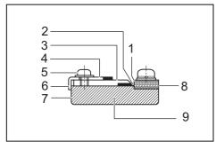
1. Inside flank of gauge plate 2. Blade edge 3. Planer blade 4. Adjusting plate 5. Screws 6. Heel 7. Back side of gauge base 8. Gauge plate 9. Gauge base
