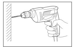
Always hold the tool only by the handle when performing an operation. Do not touch the metal part.
