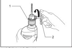
• 1. Drill chuck 2. Chuck key
