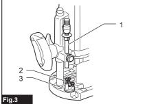
▶ 1. Stopper pole 2. Adjusting hex bolt 3. Stopper block
