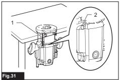
Screw M6 x 135 2. Threaded part of the motor bracket
