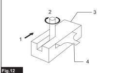
1. Feed direction 2. Bit revolving direction 3. Workpiece 4. Straight guide
