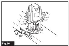
When doing edge cutting, the workpiece surface should be on the left side of the router bit in the feed direction.
