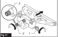
▶ 1. Thumb screw (A) 2. Thumb screw (B) 3. Scale ring
