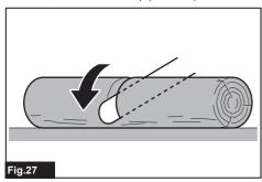
When the log is supported on one end, as illustrated, cut 1/3 the diameter from the underside (underbuck). Then make the finished cut by overbucking to meet the first cut.
