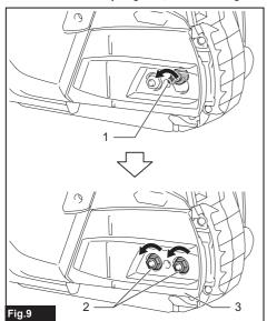
1. Chain adjusting screw 2. Retaining nuts 3. Sprocket cover
