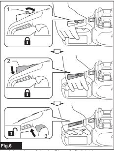
▶ 1. Lock lever 2. Lock-off lever 3. Switch trigger
