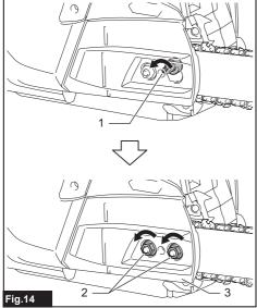
▶ 1. Chain adjusting screw 2. Retaining nuts
