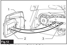
1. Sprocket cover 2. Hole 3. Bolt
