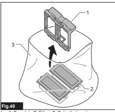
▶ 1. Top plate 2. Filters 3. Polyethylene bag
