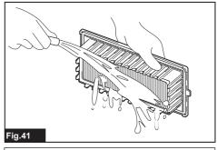
**NOTE:** Do not rub or scratch the powder filter, the prefilter and the damper with hard objects such as a brush and a paddle.
