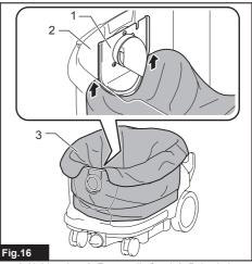
1. Holder plate 2. Front wall of tank 3. Polyethylene bag
