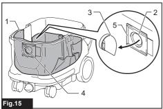
▶ 1. Filter bag 2. Cardboard opening 3. Filter bag holder 4. Dust intake 5. Edge
