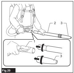
1. Bent pipe assembly 2. Ring-type extension wand
