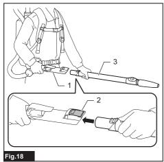
1. Bent pipe assembly 2. Button 3. Slide-type extension wand
