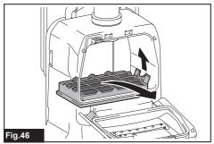
2. Beat the dust off from the HEPA filter. The HEPA filter can be washed with water. Rinse away the dust and particles on the HEPA filter every 1 or 2 month. After that, dry the HEPA filter completely in a shaded and well-ventilated place to prevent unpleasant odor or malfunctions.
