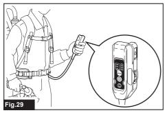
During the operation, hook the switch box on the lower belt or the D-ring.
