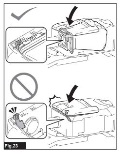
1. Unlock the lever and open the dust box cover.
