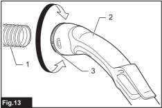
1. Hose 2. Bent pipe assembly 3. Sleeve
